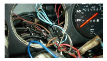
Note: It is possible that the late model Carrera have already ground to the turn signal indicator in the Tach, and the included wire setup is not needed.
