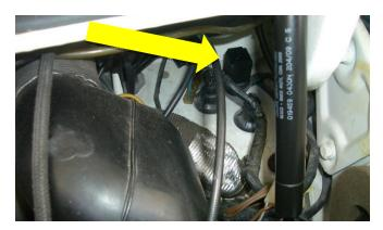
Remove the relay and replace it with the new one. **ATTENTION: Do not use the new relay with the standard bulbs, it can damage the new flasher relay.**
