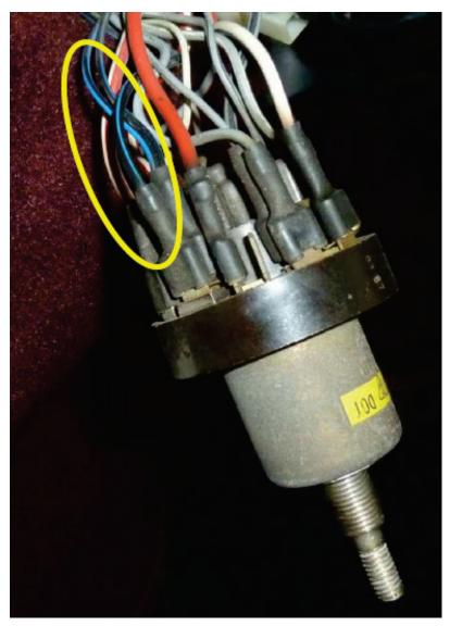
The fuse will be connected between the switch and the black-blue wire, connector No. 58a.
